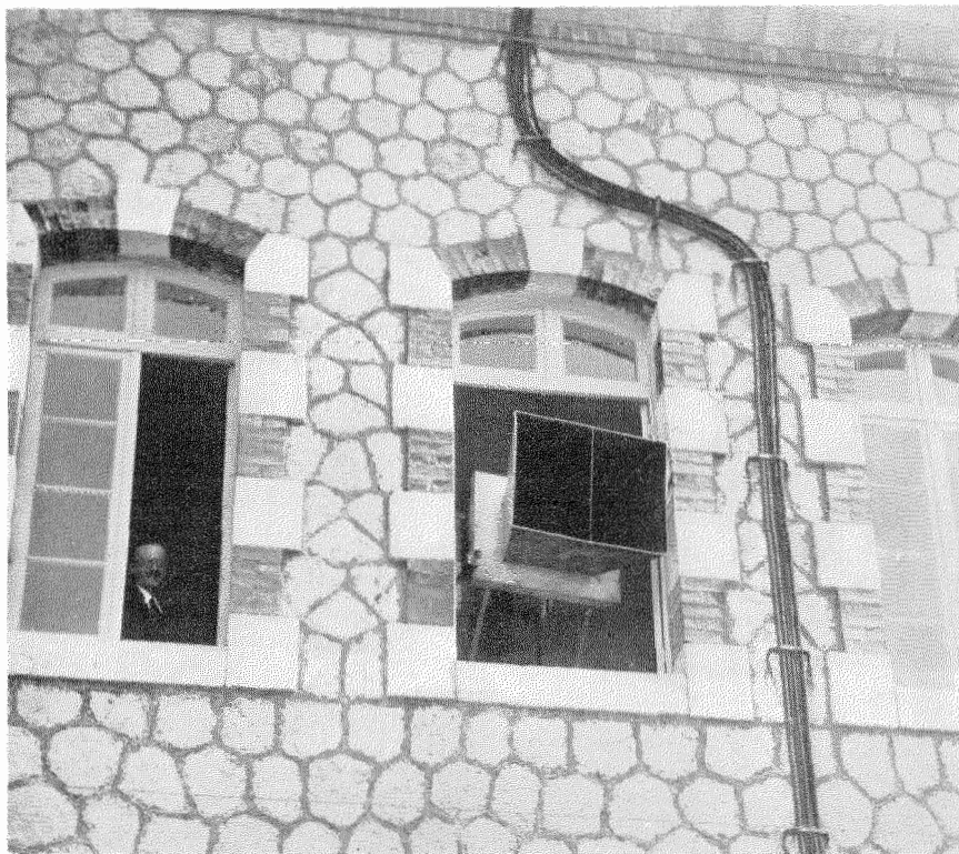
Fig. 9—3000-megacycle horn radiator used in propagation tests. The apparatus was hidden in a dismantled fort near Toulon. Colonel Labat, Chief of the Research Section of the French Signal Corps, who is standing at the window, was executed by the Germans for his underground activities.
