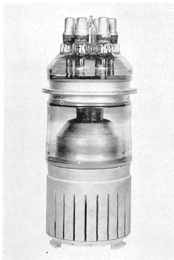
Fig. 9—8C22. At 400 megacycles, this tube will produce 500 kilowatts of peak power for pulse transmission.
