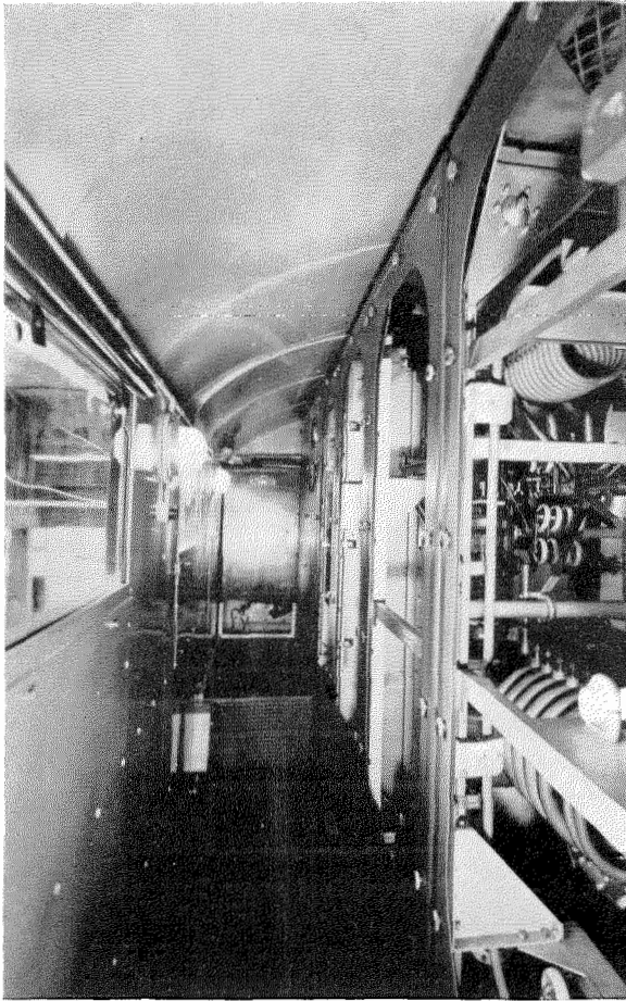
Fig. 11—Cathode-excited amplifier stage supplying a peak power of 60 kilowatts used in a 2-channel single-sideband transmitter mounted on trailers.
